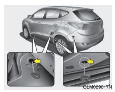
Tie-down hook (for flatbed towing) (if equipped)
