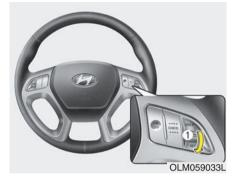
Move the lever (1) down (to SET-), and release it at the desired speed. The SET indicator light in the instrument cluster will illuminate. Release the accelerator at the same time. The desired speed will automatically be maintained.
