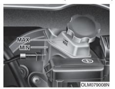
Checking the brake/clutch\* fluid level
